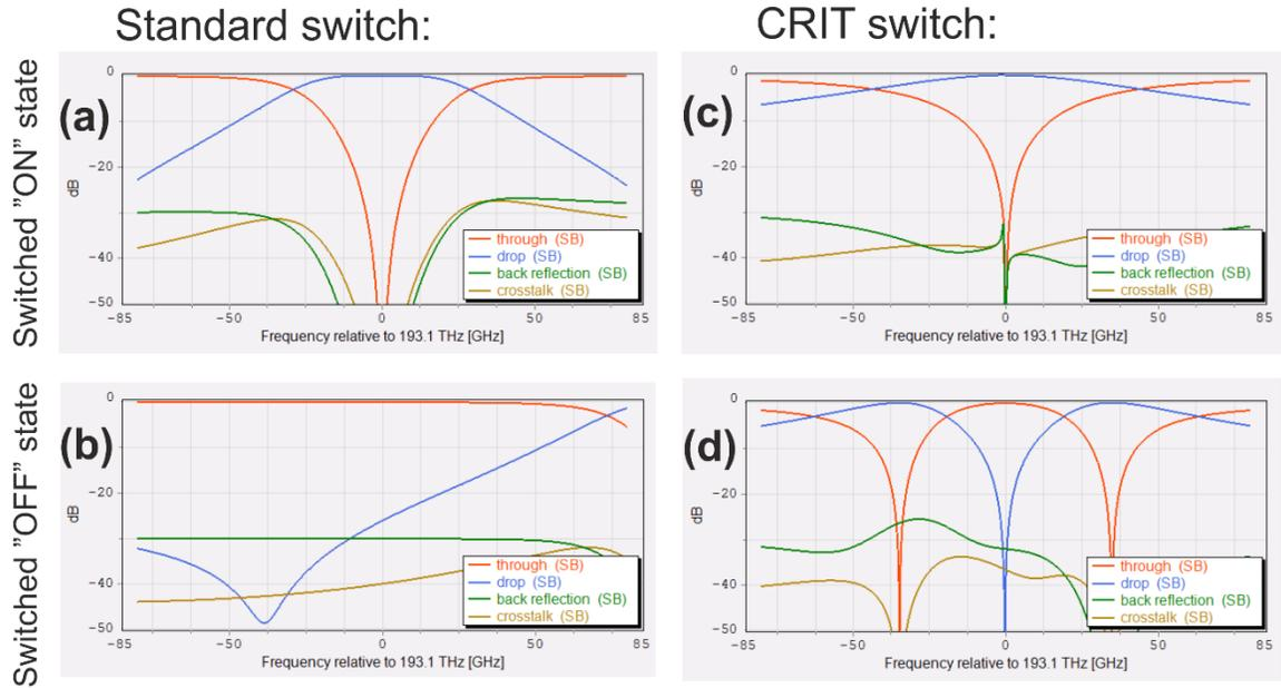
**Figure 2. Transfer characteristics of different switching mechanisms**
