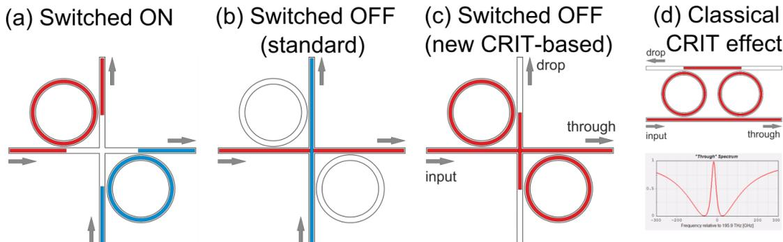
**Figure 1. 2x2 photonic switching element in different operation modes (a)-(c), two parallel micro-ring resonators exhibiting a classical CRIT effect (d)**
