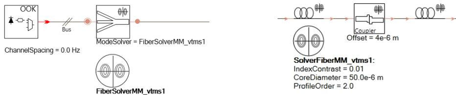
Figure 2. Combining single-mode outputs of several transmitters into one multimode signal (left) and simulation of splice-induced mode coupling (right).
