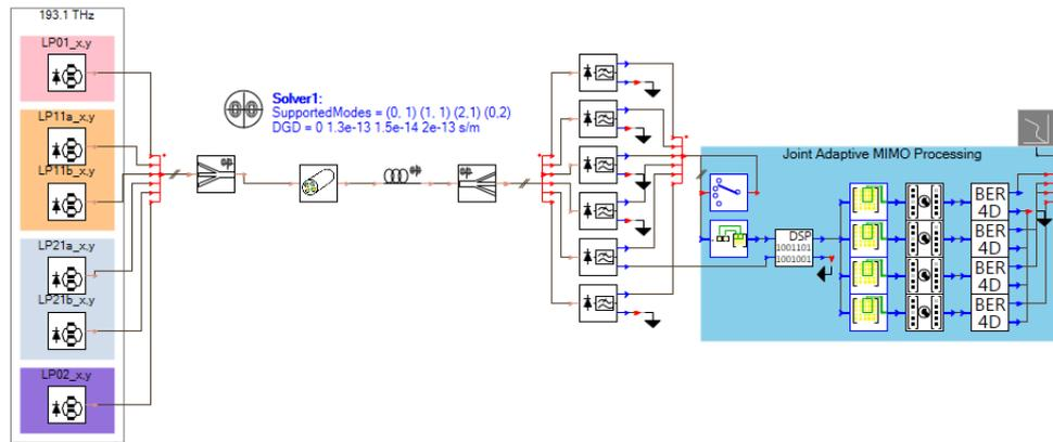
Figure 1. Simulation setup of 6 Channel SDM transmission system with MIMO equalization.
