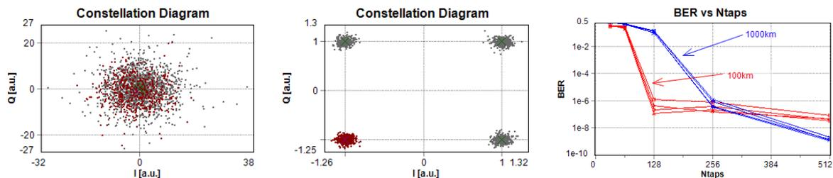
Figure 3. Exemplary constellation diagrams of uncompensated (left) and MIMO DSP-compensated (center) received signal. Plot of bit-error ratio (BER) vs. number of taps in MIMO filter for compensated receiver (right).
