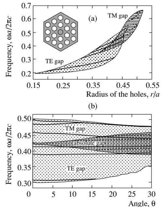
**Fig. 4.** Spectrum of localized defect modes in a triangular lattice of rotated hexagonal holes (a) as a function of the normalized hole radius  $r/a$  at a fixed value of rotation,  $\theta = 23.7^\circ$ , and (b) as a function of the rotation angle  $\theta$  for a fixed value of the hole radius,  $r = 0.43a$ . The defect is created by nonching of a single hole, as shown in the inset.
