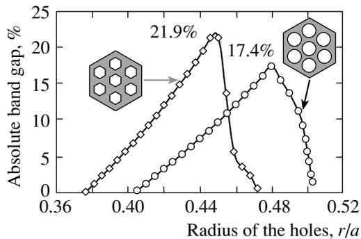
**Fig. 2.** Comparison between the absolute band gaps of two-dimensional photonic crystals created by a lattice of cylindrical (circles) and rotated hexagonal (diamonds) holes for different values of the hole radius  $r$ . For the hexagonal holes, the rotation is chosen to maximize the absolute band gap at a given radius.
