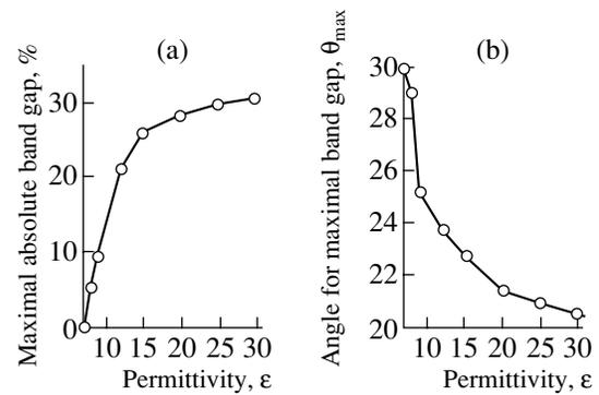
**Fig. 3.** (a) The maximum value of the absolute band gap  $\Delta\omega/\omega$  and (b) the corresponding critical rotation angle  $\theta_{\text{cr}}$  as functions of the dielectric permittivity  $\epsilon$  of the photonic-crystal material.
