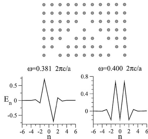
Fig. 2. Electric field  $E_n$  for two bound states supported by a  $90^\circ$  waveguide bend (shown at the top). The center of the bend is located at  $n = 0$ .
