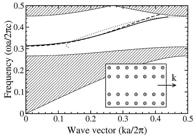
Fig. 1. Dispersion relation for the 2D photonic-crystal waveguide (shown in the inset) calculated by the supercell method<sup>3</sup> (dashed curve) and from approximate equations (5) and (6) for  $L = 7$  (solid curve) and  $L = 1$  (dotted curve). The hatched areas are the projected band structure of a perfect 2D crystal.
