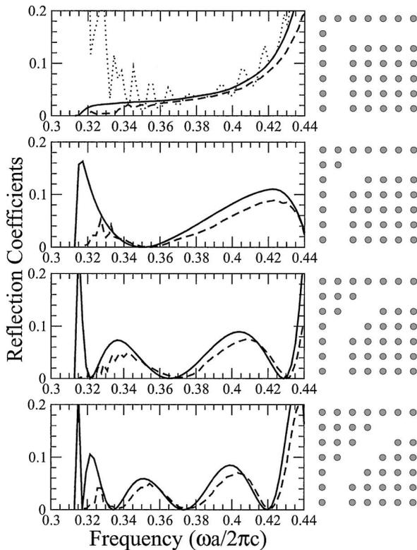
Fig. 3. Reflection coefficients calculated by the finite-difference time-domain method (dashed curves, from Ref. 5) and from Eqs. (3)–(6) with  $L = 7$  (solid curves) and  $L = 1$  (dotted curve in the top plot), for four different bend geometries.
