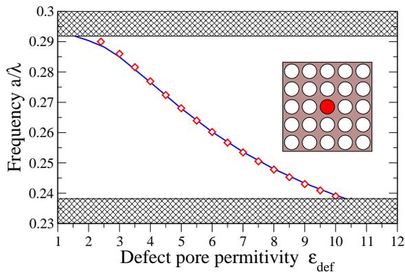
(a) Dependence of the defect frequency on  $\epsilon_{\text{def}}$  for the square lattice system.
