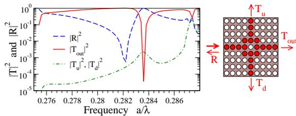
(e) Waveguide intersection square lattice.
