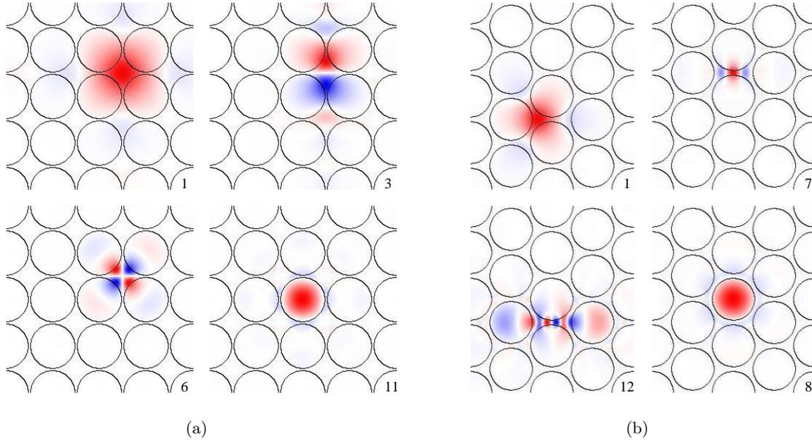
**Figure 2.** Maximally localized Wannier functions for (a) a square and (b) a triangular lattice of air pores etched into macroporous silicon. The generalized band index  $n$  is indicated in the lower right corners and the contribution of these functions to the defect mode is displayed in Fig. 3. The parameters and corresponding bandstructures of the underlying model systems are given in Fig. 1.
