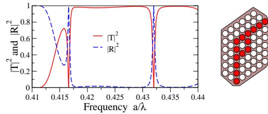
(b)  $60^\circ$  waveguide bend for triangular lattice.
