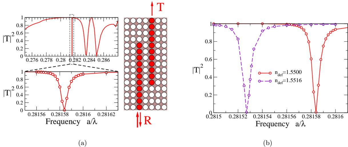
**Figure 7.** (a) Design and transmission spectrum for a folded directional coupler embedded into a square lattice of air pores. (b) Resonance dip of the transmission for different values of refractive index  $n$  of the infilled material. The parameters and corresponding bandstructures of the underlying model systems are given in Fig. 1.
