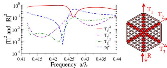
(f) Waveguide intersection triangular lattice.
