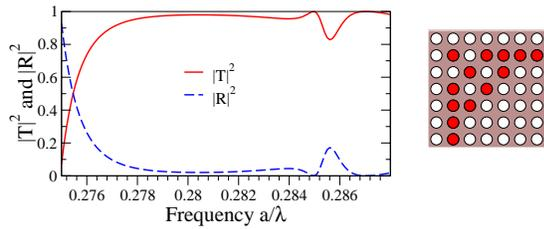
(a)  $90^\circ$  waveguide bend for square lattice.
