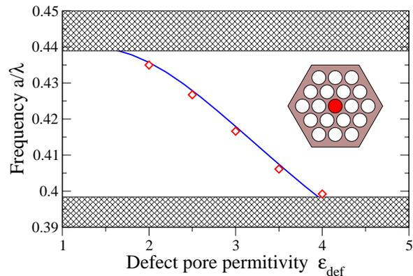
(b) Dependence of the defect frequency on  $\epsilon_{\text{def}}$  for the triangular lattice system.
