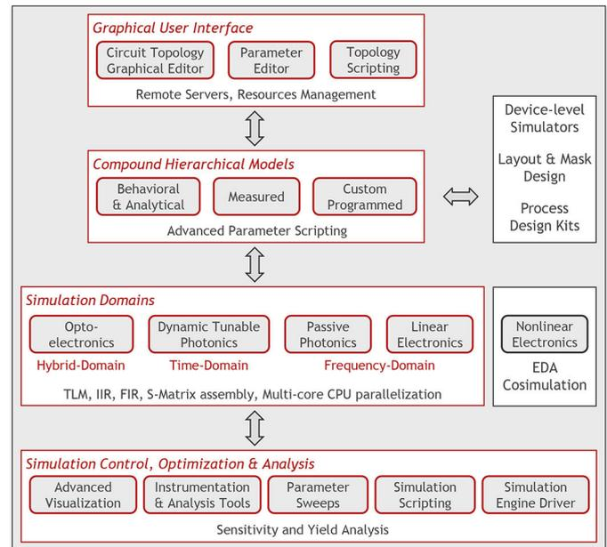
**Figure 1.** Organization of VPIcomponentMaker Photonic Circuits, a circuit simulator addressing the complex requirements of an automated design framework for integrated photonic and optoelectronic circuits. TLM: Transmission line model. IIR: Infinite impulse response. FIR: Finite impulse response. S-Matrix: Scattering matrix. CPU: Central processing unit.
