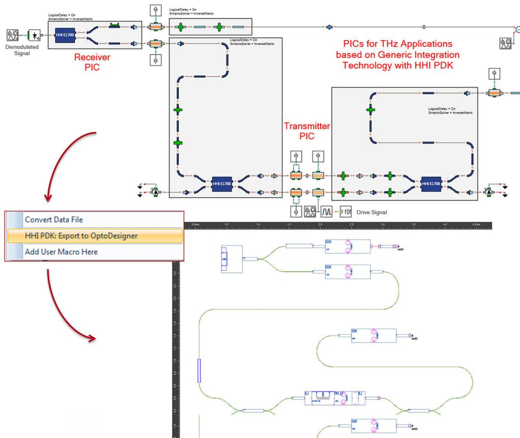
**Figure 2.** Photonic integrated circuits (PICs) for THz generation and detection. The photonic circuit design, constructed in VPIcomponent-Maker Photonic Circuits using specialized building blocks adhering to the process design kit (PDK) of the Fraunhofer Heinrich-Hertz Institute (HHI) foundry (top), is exported for layout design in Phoenix OptoDesigner (bottom). SOA: Semiconductor optical amplifier. BJ: Butt joint. PM.CI: Current-injection phase modulator.
